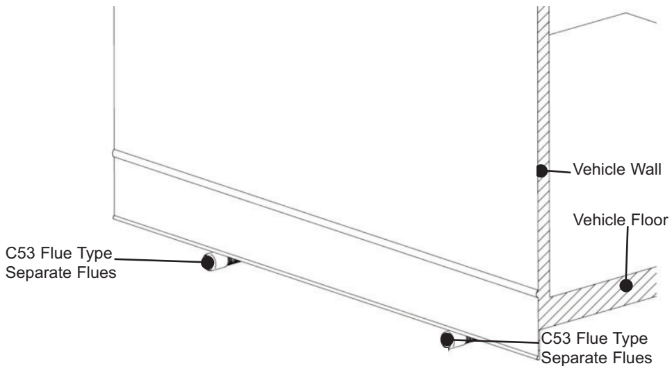
Fig. 19 Flue Type for Standard Installation
